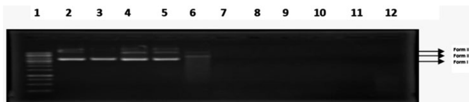
Figure 9. Cleavage of SC pBR322 ( 0.5 \mu\text{g } \mu\text{L}^{-1} ) \text{Ni(L5)}_2 at different concentrations in Tris-HCl buffer pH (7.2) for 2 h at 37^\circ\text{C} . Lane 1: DNA ladder; Lane 2: DNA + \text{H}_2\text{O}_2 ; Lane 3: DNA + \text{Ni(L5)}_2 (1 mM) + DMSO; Lanes 4–12: DNA with increasing the concentrations of \text{Ni(L5)}_2 (0.1–1 mM) + \text{H}_2\text{O}_2 + 1% DMSO.
